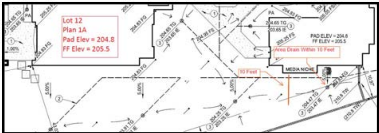
Figure 5 Example of Area Drains Used Within 10 Feet of Foundations When Slope < 5% in 10 Feet.
